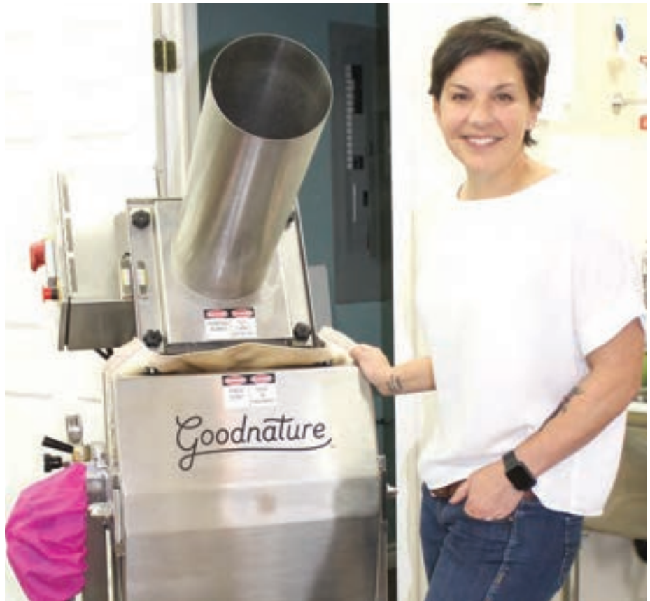
Glow Juicery PEI has the only cold-pressed commercial juicer in the Maritimes. Fruit and vegetables are tossed down the top chute to be ground into juice, which is filtered out below. Melissa Heald photo
